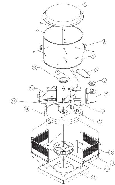
PARTS LIST LEGEND Description Qty. Description No. Qty. No. 0 Bag of Hardware (not shown) 1 9 **Disconnect Device** 1 2 1 Hood Top 1 10 Bird Screen \*\* 2 Hood Fastener Conduit 11 1 Curb Base and Orifice 3 Windband 1 12 1 4 Motor Base 1 13 Wheel\* 1 5 Drive Belt\* \*\* 14 Pan Separator 1 Motor Sheave\* 15 Bearing Cap 6 1 1 7 Motor\* 1 16 Fan Sheave\* 1 8 Windband Bracket 2 99 Shaft and Bearing Assembly 1
